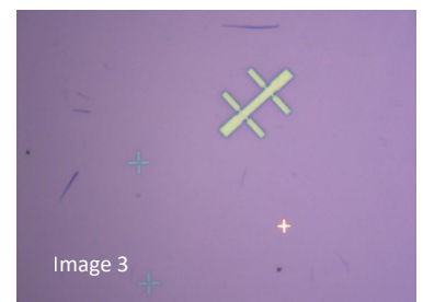
Image 1: Graphene transferred onto an Si/SiO 2 substrate. A photoresist Hall bar pattern (yellow) is formed on top of the graphene.
