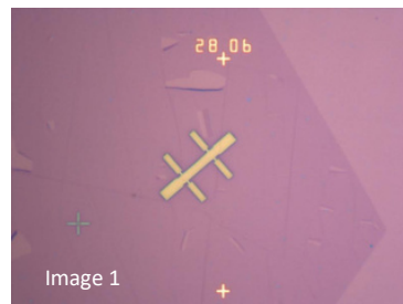
Image 1: Graphene transferred onto an Si/SiO 2 substrate. A photoresist Hall bar pattern (yellow) is formed on top of the graphene.
