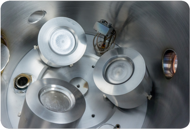
3 magnetron sputtering sources inside the chamber with quartz crystal sensor head
