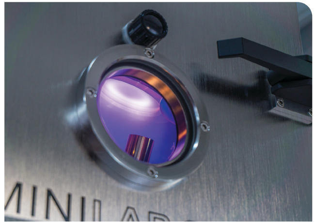
Viewport with integrated shutter to protect the window when not in use.
