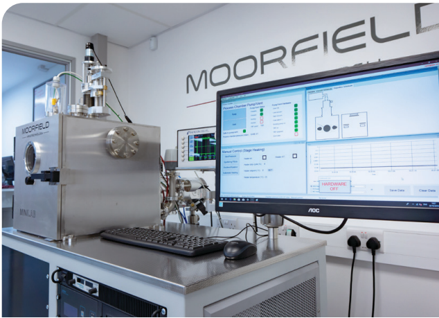
PC user interface for system control and monitoring. Manual and automated modes of operation.
