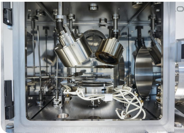
MiniLab 070 tool with sputter-down configuration
